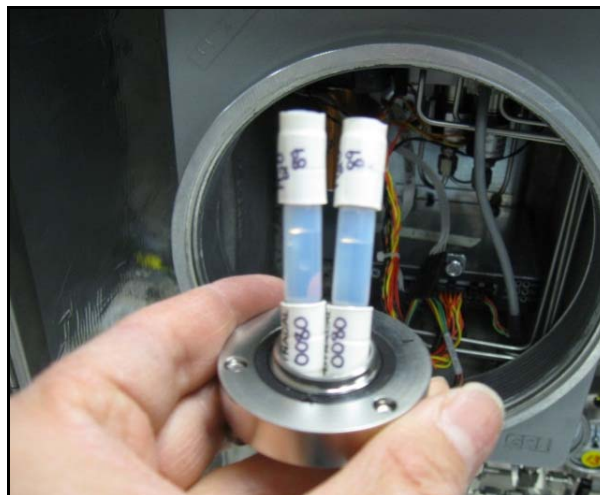
Figure 85: Water in Permeation Tubes
