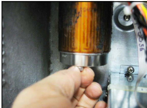
Figure 88: Tightening the Bolts
