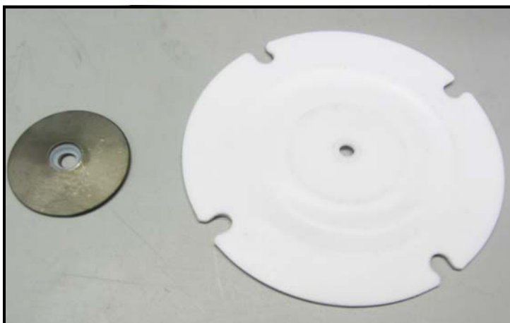
Figure 78: Installing the New Diaphragm and Clamping Plate
