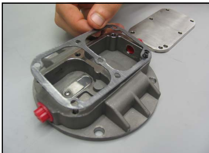
Figure 76: Installing the New Valve Cover Gasket
