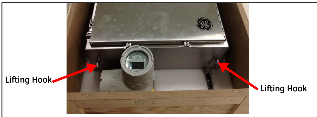
Figure 3: Lift Aurora Trace up Above the Ground from the Two Hooks Shown
