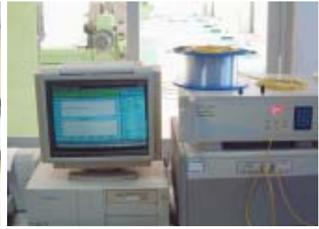
Chromatic Dispersion of Optical fiber tester
